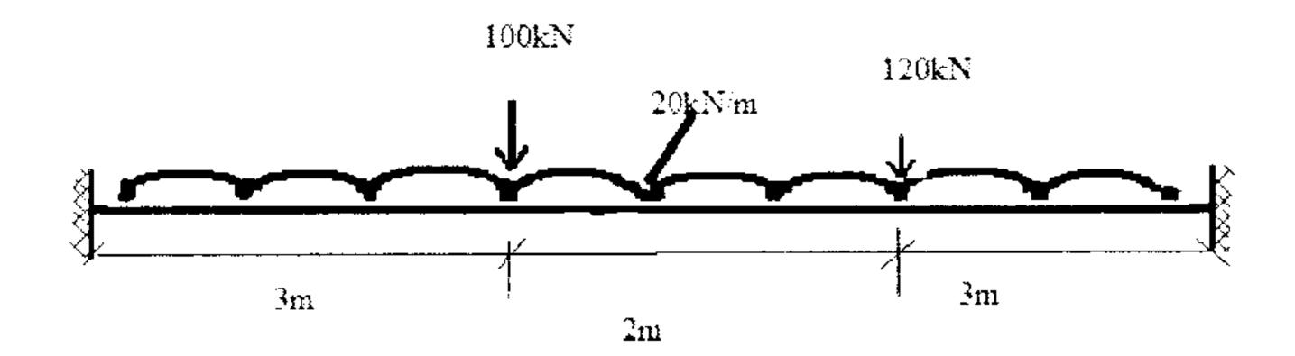
4. Analyse the continuous beam as shown in figure below.Adopt Clapeyron's theorem of three moments method. Also Draw Bending Moment Diagram.14 M
