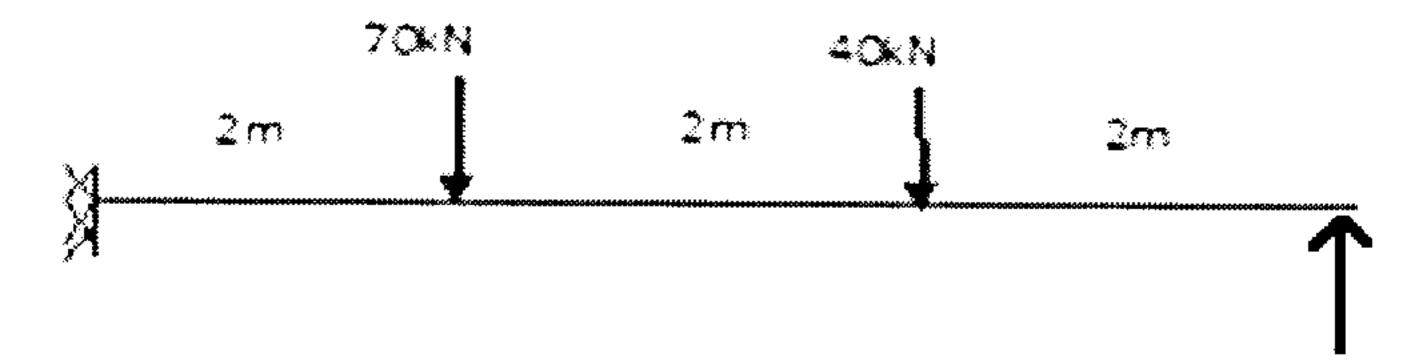
3. Draw the bending moment and Shear force Diagram for the structure shown below.
